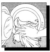
Open the door by pulling the catch outwards. Load the items to be washed one at a time and close the door.
